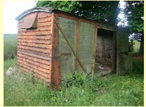
Library photo of a similar Vanfit goods van body in a similar condition
